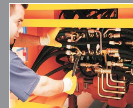
Separated hose system ensures economical, quick service and short repair period.
